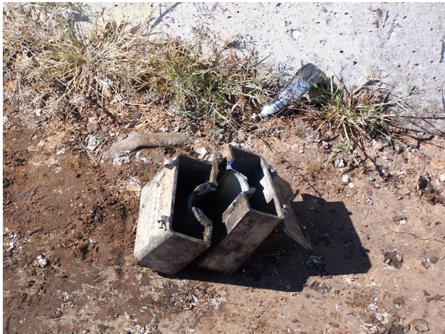
Lubricator Box that failed causing the rod string to fall.
